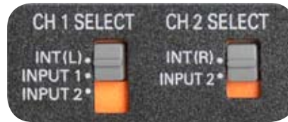
Two switches behind LCD panel
